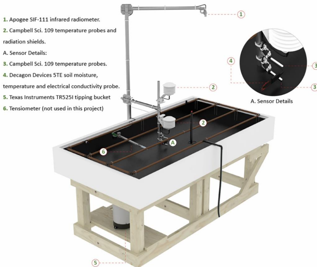
Figure 1: Example test roof and instrumentation of a GREEN test roof. Figure modified from original GRIT lab design schematic generated by Benjamin Matthews (2012). Reproduced with permission.
